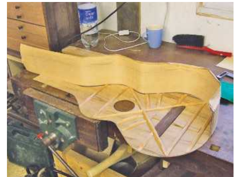
▲ Pic.15 Plane the bottom edge of the side flat so it will mate perfectly with the soundboard
